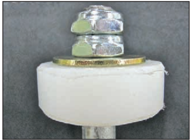
When pucks are replaced, heavy nut will be replaced by another low profile nylock nut. When two low profile nuts are present there must be at least one thread of bolt sticking out.
