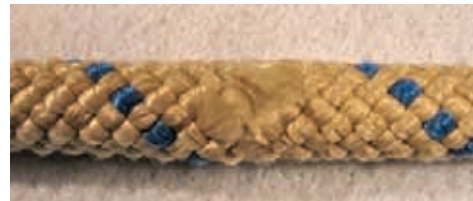
Rope is fraying. Individual picks not visible. Rope is NOT safe for use.
