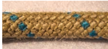
Used rope. Note the “fuzzy” appearance, however, individual picks are still easily distinguishable. This rope is safe to use.
