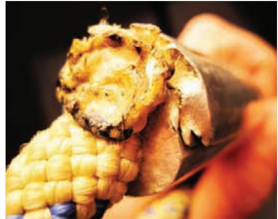
A Crack in this ferrule goes all the way through to the rope and is only visible looking down ferrule.
