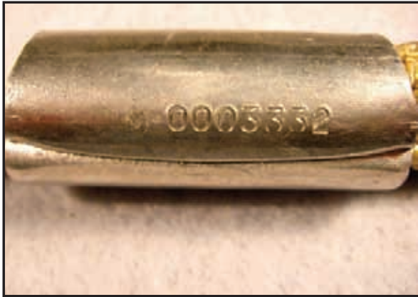
This ferrule is good. Serial number is present and easily visible.
