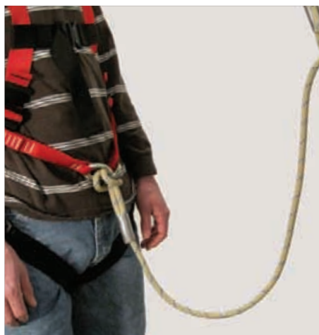
Sling line length incorrect - TOO LONG
