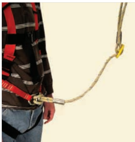
Sling line length - Correct
