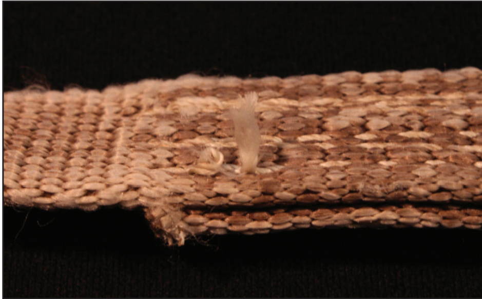
Piece of thread sticking out where it has been cut after sewing. This is ok as long as the stitching does not unravel if this piece is pulled on.
