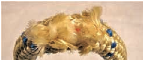
Major cut in rope exposing the core. Rope is NOT safe for use.
