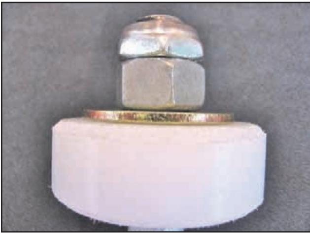
Bolt must be at least flush w/nylock nut or have threading sticking out.
