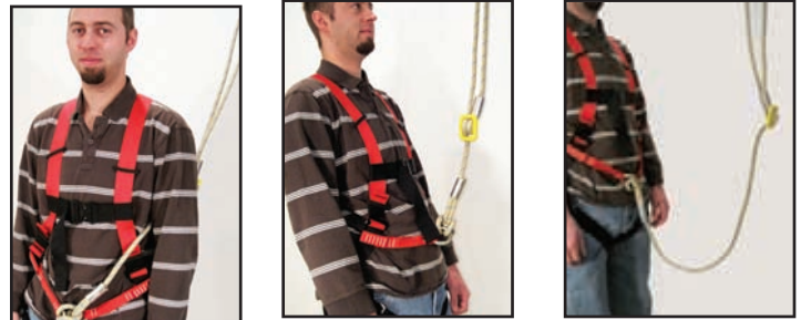
SLING LINE - INCORRECT
