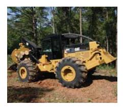
**Box-Section Construction.** Caterpillar designed and manufactured box section structures set the industry standard for reliable, durable main frames. Extensive computer analysis and field-testing resulted in the design of the 525C.
