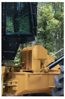
Hydraulic Winch. The 525C features an electronically controlled hydraulic winch for grapple applications, replacing the mechanical winch. The hydraulic winch improves application flexibility by allowing the tractive effort to be used while winching, and eliminating the continuously rotating driveshaft.
