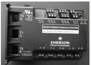
Figure 48 - Variable Capacity Compressor Controller
