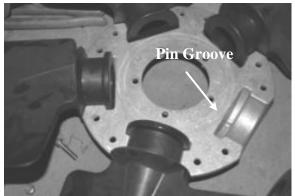
Figure 38 - Pin Groove Location
