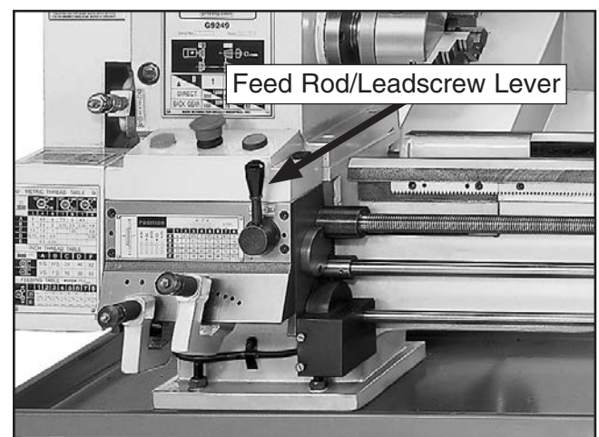
Figure 16. Feed rod/leadscrew lever in center (neutral) position.
