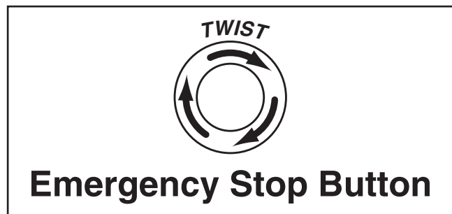
Figure 17. Resetting the emergency stop button.
