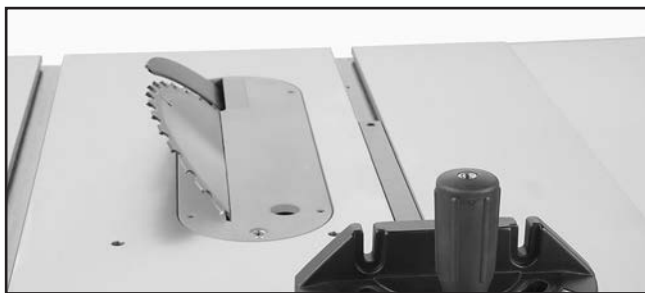
Figure 53. Blade tilted to 45° for bevel cutting on a typical table saw.
