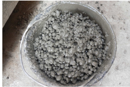
Picture 6: Expanded Clay meshed with cement
