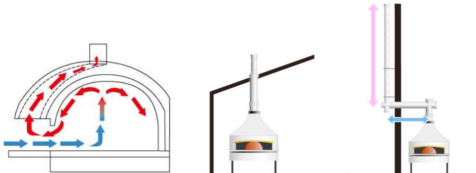
Picture 4: Air circulation into the oven and example of typical chimney installation schemes
