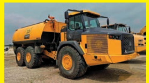
2015 JOHN DEERE 410E SN:670286 6x6, powered by John Deere diesel engine, equipped with Cab, air, heat, Niece 8,000 gallon tank, side and rear spray heads, water cannon, 29.5R25 rubber.
