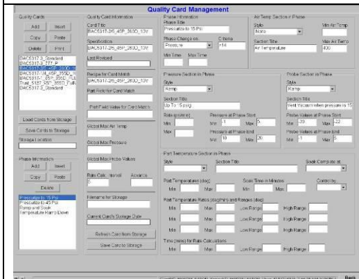
Automatic quality system designed to analyze data per spec. and provide Pass/Fail results.
